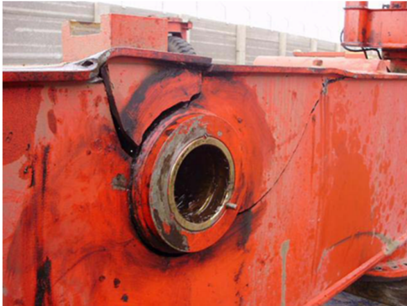
1. Equalizer beam web under center equalizer pin
